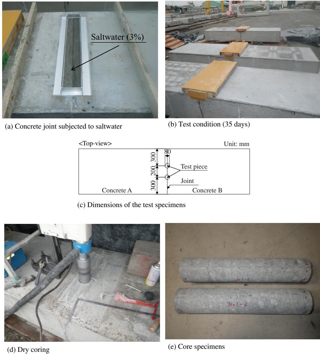
Fig. 10. Saltwater permeability test: (a) Concrete joint subjected to saltwater; (b) Test condition (35 days); (c) Dimensions of the test specimens; (d) Dry coring; (e) Core specimens.
