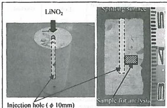
Fig. 2 The extraction position of the sample for analysis.
