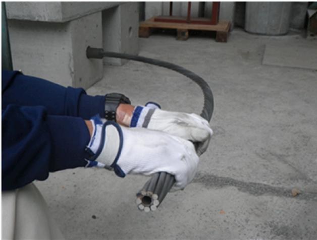
(a) Hollow corrugated pipe covered with steel-wire cables
