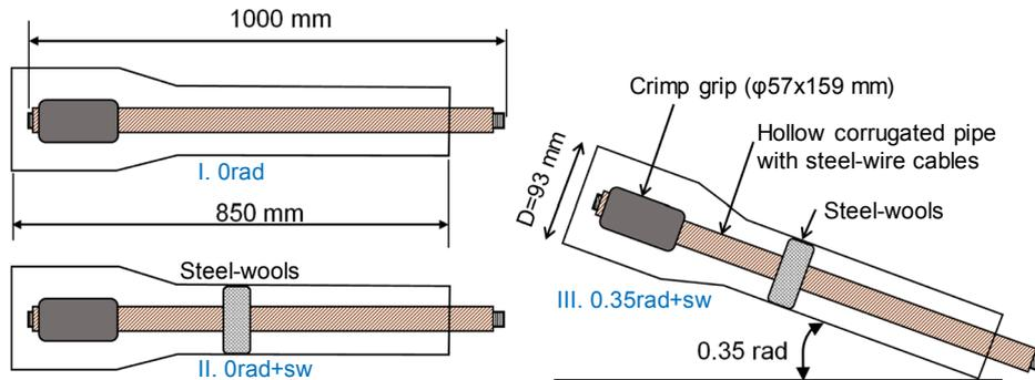
(c) Schematic of test parameters
