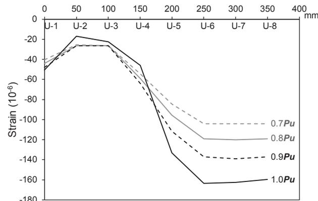
(b) Axial strain of concrete
