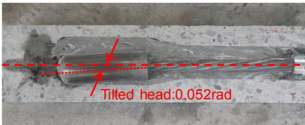
Fig. 15. Saw-cut anchorage embedding the flexible tendon.
