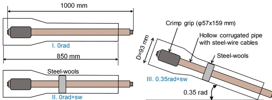
(c) Schematic of test parameters
