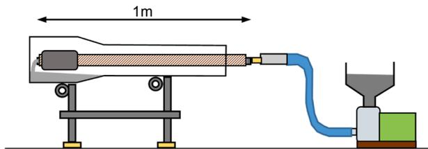
(b) Schematic of grouting test
