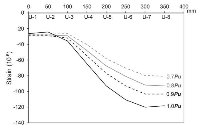
(b) Axial strain of concrete
