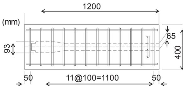
(e) Rebars arrangement -side view-
