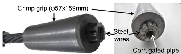
Fig. 4. Crimp grip for flexible tendon.
