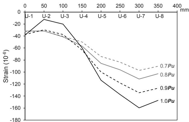
(b) Axial strain of concrete
