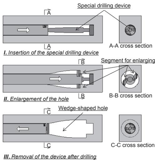
(a) Drilling for a wedge-shaped anchor
