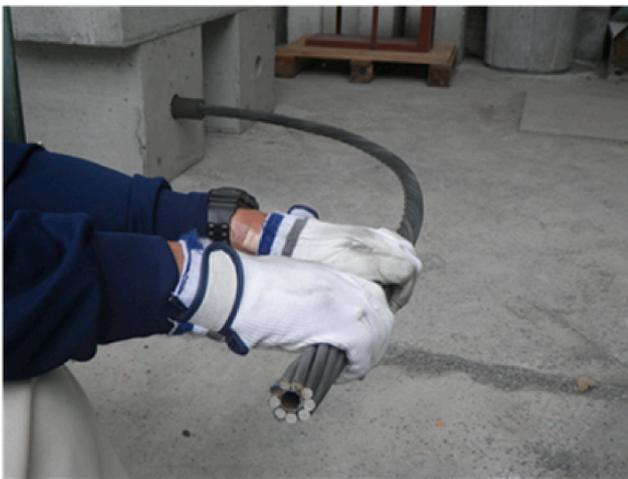
(a) Hollow corrugated pipe covered with steel-wire cables
